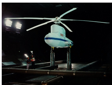
Figure 1. Sikorsky bearingless rotor mounted in the NASA Ames 40-by 80-Foot Wind Tunnel.
