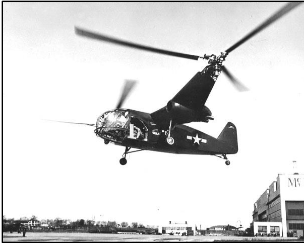
Figure 1. McDonnell XHJD-1 Whirlaway side-by-side rotors helicopter (Courtesy of Boeing)
