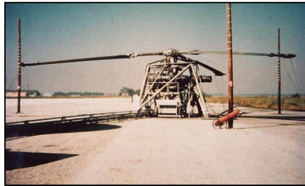
Figure 6. The MAC designed and built hot whirl test stand at Smartt Field, north of St. Louis (Courtesy of Bob Head via Ken Bartie, Boeing).
